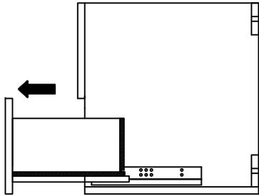
2. Pull out the bottom of the rail plastic insert
