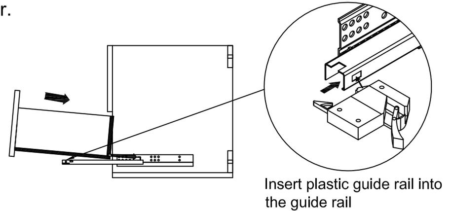
2. Align the drawer rear hole with the rear hook of the guide rail.
