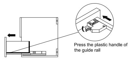
2. Pull the drawer out of the rear hook of the guide rail.
