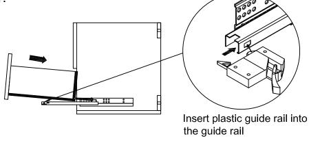
2. Align the drawer rear hole with the rear hook of the guide rail.
