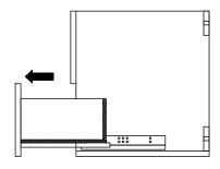
2.Pull out the bottom of the rail plastic insert
